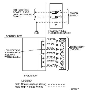
Fig. 4—50GL High- and Control-Voltage Connections
